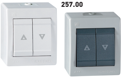
257.00 257.1A Taster sklopka za roletne 10A/250V~ IP44 Rolling shutter push-button switch 10A/250V~ IP44 • Dve taster sklopke za direktno pokretanje elektromotora za podizanje i spuštanje roletni, • Blokada koja sprečava istovremeno kretanje u oba smera • Two push-button switches for direct activation of rolling shutters lifting and lowering electric motor • Interlock of movement in both directions simultaneously
