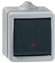
289.1A Sklopka jednopolna sa indikatorom 16AX/250V- Single-pole switch with indication 16AX/250V- • Indikacija svetli kada je sklopka isključena • Indication turns on when the switch is off
