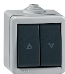
287.1A Taster sklopka za roletne 10AX/250V- Rolling shutters switch 10AX/250V- • Dve taster sklopke za direktno pokretanje elektromotora za dizanje i spuštanje roletni, • Blokada mogućnosti uključanja kretanja istovremeno u oba smjera • Two push-button switches for direct activation of rolling shutters lifting and lowering electric motor • Locking of movement switching-in possibilities simultaneously in both directions
